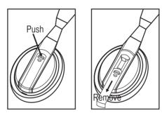
2. Insert the battery by pressing the minus pole of the battery against the spring on the battery compartment until the plus pole can slide into the battery compartment. The battery should snap into place.
